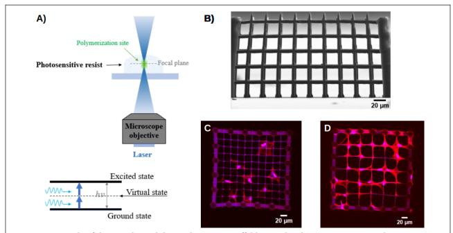
Fig. 1: A) Principle of the two-photon lithography. B) 3D scaffold printed with Ormocomp resist, whose pore size is 20  $\mu$ m and fibre size is 5,3 +/- 0,3  $\mu$ m in any direction. C-D) NIH 3T3 fibroblasts grown in scaffolds whose fibre diameter is 3  $\mu$ m and pore size is 20  $\mu$ m (C) or 40  $\mu$ m (D). the cells are labelled for actin cytoskeleton (red) and nuclei (blue). Cell morphology and area appear sensitive to pore size in this range of parameters.
